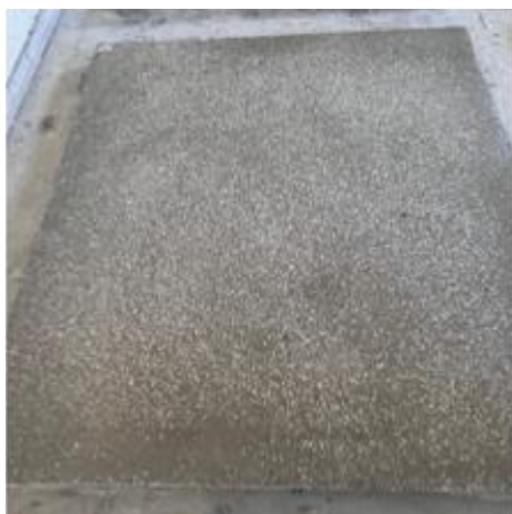
Four floor samples were tested between Tsumeb and Aris aggregates, before the final finish was selected, balancing heritage sensitivity, technical requirements and cost.
