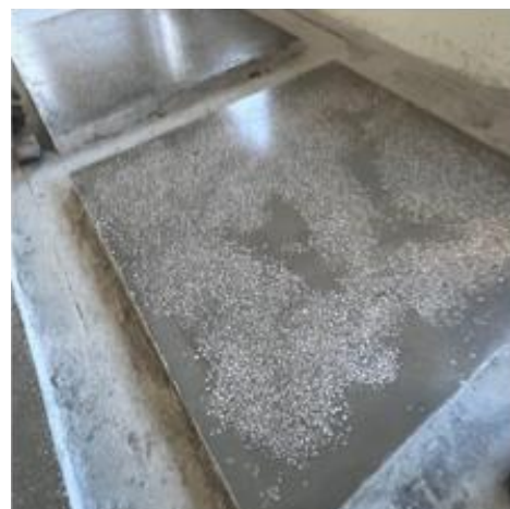
Four floor samples were tested between Tsumeb and Aris aggregates, before the final finish was selected, balancing heritage sensitivity, technical requirements and cost.
