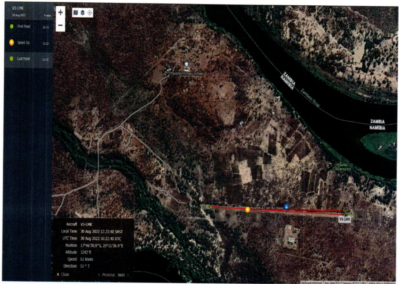
Figure 3: Picture showing the take-off from Impalila Island and the data pertaining to the take-off maneuver performed by the aircraft before it crashed.
